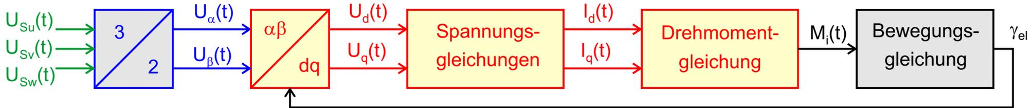
$$\text{allgemein: } P_i(t) = \frac{3}{2} \cdot \text{re} \{ \underline{U}_{idq} \cdot \underline{I}_{sdq}^* \} = \frac{3}{2} \cdot (U_{qi} \cdot I_q + U_{di} \cdot I_d) \quad \text{für } \underline{U}_{idq} = U_{di} + jU_{qi} \quad \text{und } \underline{I}_{sdq} = I_d + jI_q$$
